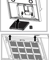
Assembly: Secure the activated-carbon filter first in the back using the hood's metal tabs and then in the front by pressing the two levers.
